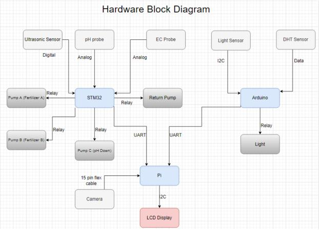
Figure A1: Hardware Block Diagram [12]
