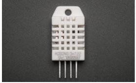
Figure 12: Temperature and Humidity Sensor [13]
